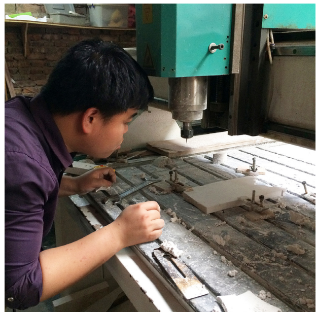
Fig 2. CNC Milling of plaster slab for making a low relief drop mould, Jingdezhen, China, 2017 Photo: Paul Leathers
