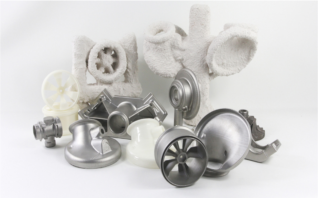
Fig 8. Polymaker Polycast™ models with stainless steel castings Photo: Polymaker Industrial
