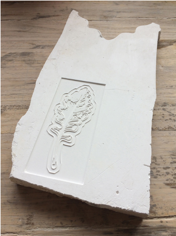
Fig 3. CNC Milled plaster drop mould Photo: Paul Leathers
